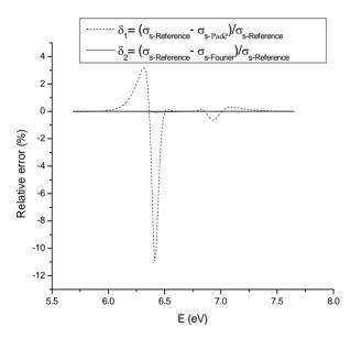
Figure 12. Relative error for average scattering cross sections of the  $E_0$  = 6.67 eV resonance for the  $^{238}\rm{U}$  isotope and T = 1500 K.
