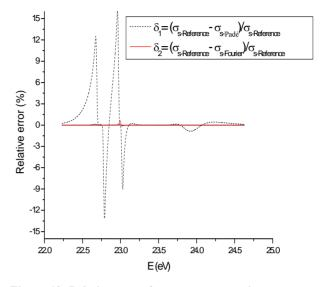
Figure 13. Relative error for average scattering cross sections of the  $E_0 = 23.43$  eV resonance for the  $^{232}$ Th isotope and T = 1500 K.
