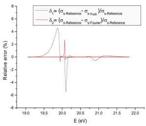
Figure 14. Relative error for average scattering cross sections of the  $E_0 = 20.45$  eV resonance for the <sup>240</sup>Pu isotope and T = 1500 K.
