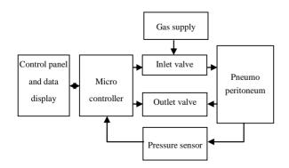
Figure 1. Block diagram of the electronic pressure control system.
