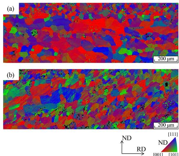
**Figure 3.** Orientation color maps obtained by EBSD after hot strip annealing and one-pass ECAP.
