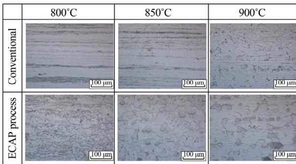
**Figure 6. Microstructures by optical microscopy after final annealing showing partially and fully recrystallised states in (a) Conventional and (b) ECAP processes.**
