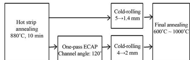
**Figure 2.** Flow diagram of fabrication process of cold-rolled and annealed sheets by conventional process (upper) and ECAP process (lower).
