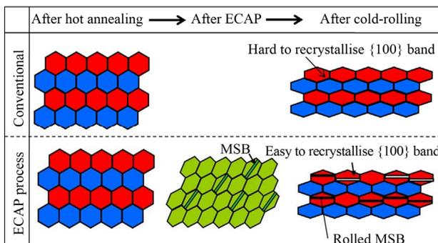
**Figure 9.** Schematic diagram showing fragmenting process by embedding grain-scale microshear bands in extended {100}//ND grains. Fragmented {100}//ND grains become readily recrystallised on subsequent annealing.
