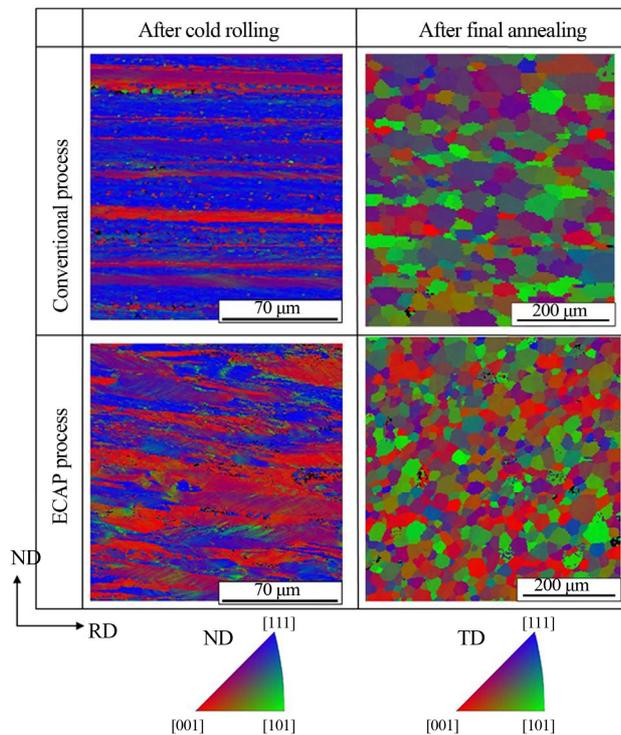
**Figure 4.** Orientation color maps observed from TD direction after cold-rolling and the final annealing. Orientation is expressed in terms of ND and TD directions, after cold-rolling and annealing, respectively.
