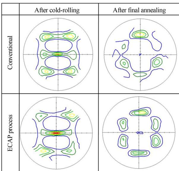
**Figure 7. {100} pole-figures showing textures after cold-rolling and final annealing in conventional and ECAP process.**
