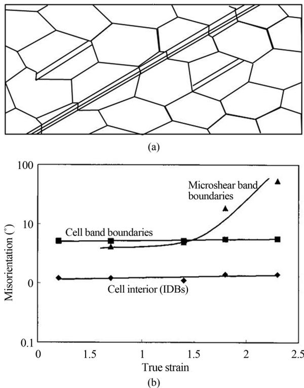
**Figure 8.** (a) Schematic diagrams of shear band and grain-scale microshear bands; (b) Effect of strain on the mean misorientations of cell, microshear bands in Al-0.1% Mg [27].
