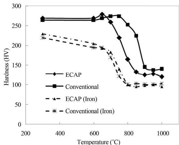
**Figure 5.** Influence of annealing temperature on hardness of ECAP and the conventional processes. Data of pure iron by same processing are also shown for comparison.
