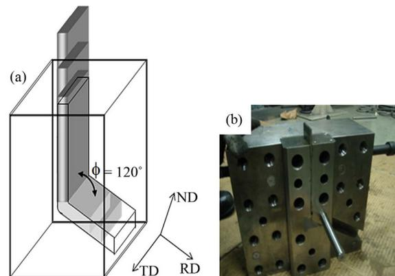
**Figure 1.** (a) Schematic diagram of ECAP processing. ND, RD and TD directions are defined with regard to the sheet; (b) Photo of ECAP die.
