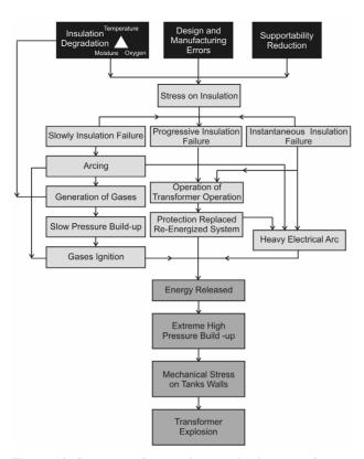
Figure 12. Sequence of event that can lead to transformer explosion (adapted from Ronningen [4]).
