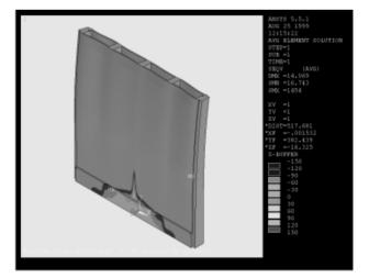
Figure 7. Von Mises tension test on firewall after 60 minutes.
