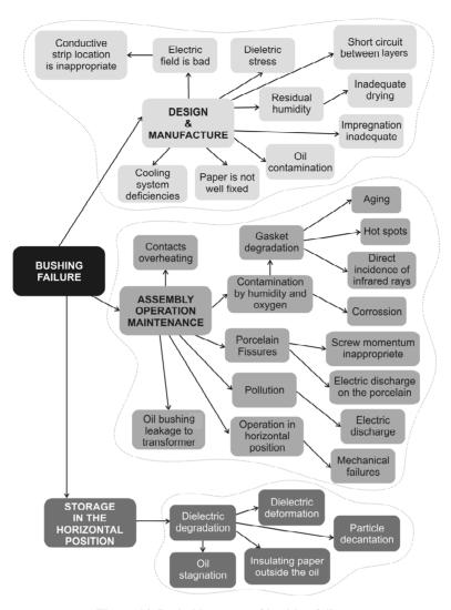
Figure 14. Probable causes of bushing failure.
