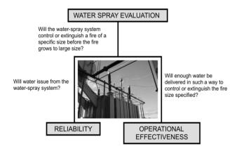
Figure 10. Evaluation of water-spray system.
