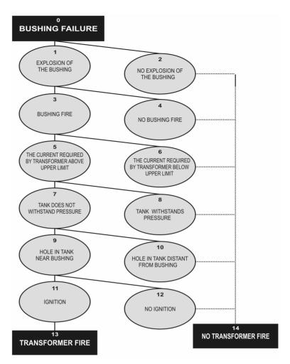
Figure 15. Bushing failure.
