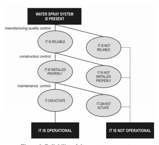
Figure 9. Reliability of the water-spray system.
