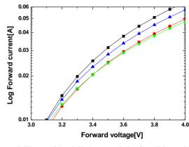
Figure 4. The semi-log I-V characteristics for all investigated LEDs at high forward bias.
