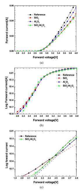
Figure 3. The linear and semi-log I-V characteristics for all investigated LEDs at forward bias (a) and (b). To clearly see the difference, we compared the I-V curves for only two LEDs in (b) of the figure with non-passivated LED and the  $SiO_2/Al_2O_3$  double dielectric passivated LED.
