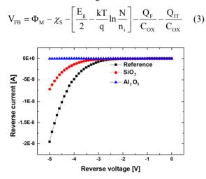
Figure 6. The LED with  $Al_2O_3$  layer exhibits at least two and three orders lower in leakage current compared to that with SiO<sub>2</sub> layer and without dielectric layer, respectively.
