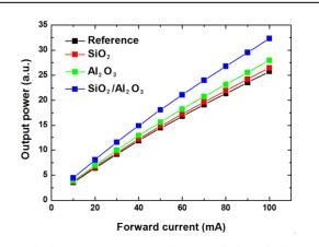
Figure 7. The output power characteristics of the nonpassivated, the  $SiO_2$ -passivated, the  $Al_2O_3$ -passivated, and the  $Al_2O_3/SiO_2$ -passivated LED. The output power of the  $Al_2O_3/SiO_2$ -passivated LED exhibits about 25% higher than that of the non-passivated LED.
