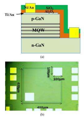
Figure 1. The schematic of the LED configuration investigated in this work (a); and the fabrication of the 430  $\mu$ m × 430  $\mu$ m size real LED chip (b).
