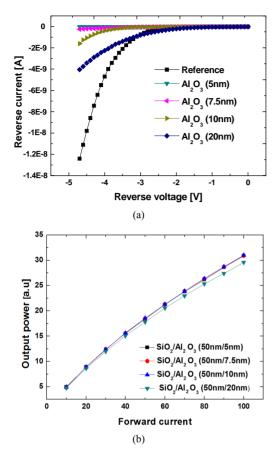
Figure 2. The the leakage current characteristics (a) and the output power characteristics (b) of the SiO<sub>2</sub> (50 nm)/Al<sub>2</sub>O<sub>3</sub> (5 nm), SiO<sub>2</sub> (50 nm)/Al<sub>2</sub>O<sub>3</sub> (7.5 nm), SiO<sub>2</sub> (50 nm)/Al<sub>2</sub>O<sub>3</sub> (10 nm), and SiO<sub>2</sub> (50 nm)/Al<sub>2</sub>O<sub>3</sub> (20 nm)-passivated LEDs, respectively.
