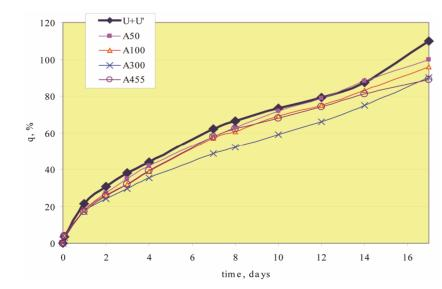
Figure 2. The curves of swelling (11°C) in the concentrated HNO<sub>3</sub>, samples with 2 wt% of unmodified NS.
