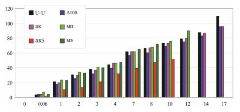
Figure 4. Histogram of swelling of the samples with 2 wt% (for ak5—5 wt%) A-100 and its modified forms (black column—the average value for the unfilled samples).
