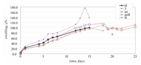
Figure 5. Swell curves in c.HNO<sub>3</sub> (25°C) for EP-templates with 5 wt% of silica: H: unfilled; 3: aerosil A-300; ak: A-300/mod.acrylsilane A174 (monolayer); akB: A-300/mod.acrylsilane A174 + olygoacrilate Bis-GMA; B: A-300/mod.olygoacrilate Bis-GMA (monolayer).
