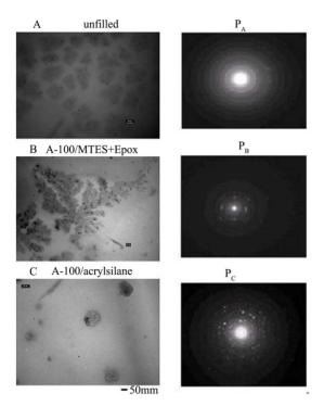
Figure 7. Photomicrographs and X-ray of unfilled sample polyepoxides (A) filled with 2% aerosil A-100, modified MTES and ED-5 (B) and modified by acrylate silane A-174 (C).
