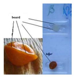
Figure 6. The visual shape of EP-template "B"—initial thick (up) and after 12 days in c.HNO<sub>3</sub> (ball-like).
