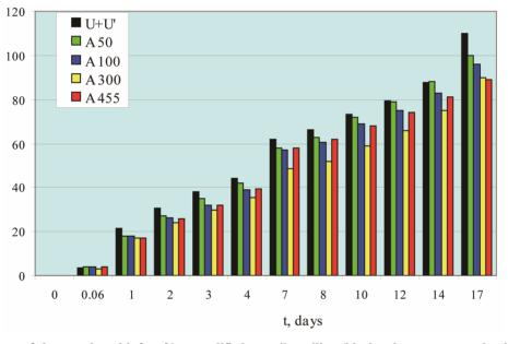
Figure 3. Histogram of the samples with 2 wt% unmodified aerosil swelling (black column—averaged values—of q for the unfilled samples).
