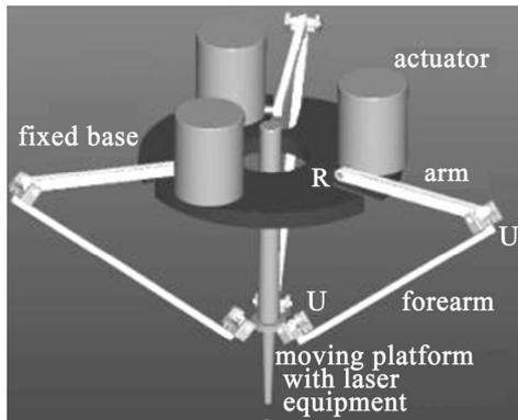
Figure 5. Three RUU kinematic chains usage in delta robot for laser cutting [13].
