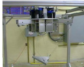
Figure 12. Cable-suspended robot designed and assembled at University of Delaware [20].
