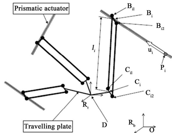
Figure 9. Use of linear drives in delta structure for 3-axis parallel machine tool [17].
