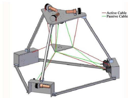
Figure 13. Seven-cable robot with 6-cable passive metrology (2004) [21].
