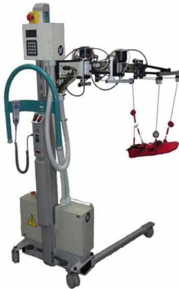
**Figure 19. MariBot—a platform for upper arms using cable-based parallel manipulator [28].**
