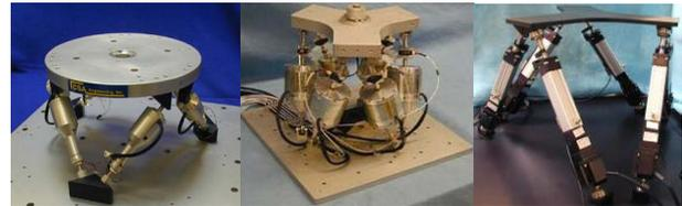
Figure 7. Hexapods using piezoelectric, electromagnetic and motor-driven screw actuators [15].
