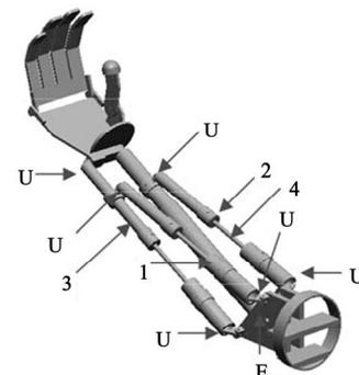
**Figure 17.** Elements of prosthesis using parallel topology with 3 line actuators [26].
