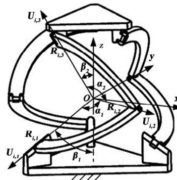
**Figure 4.** Three DOF spherical parallel manipulators [12].
