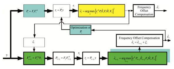
Figure 5. Interference elimination and frequency offset estimation in interleaved subcarrier allocation scheme by using SSP method.
