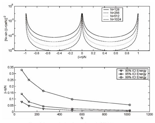
Figure 3. Inter-carrier-interference factors in OFDMA systems.
