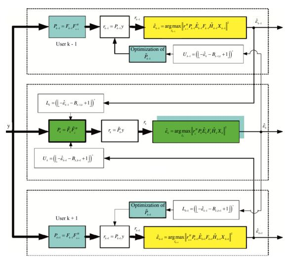
Figure 4. Interference elimination and frequency offset estimation in block-based subcarrier allocation scheme by using RRP method.
