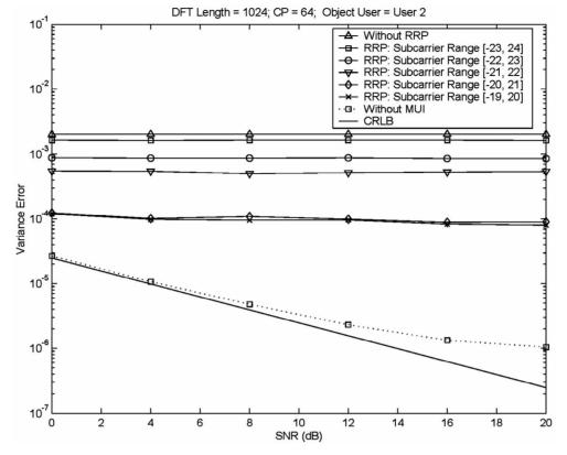
Figure 7. Frequency offset estimation with the help of heavy MAI elimination by using RRP.
