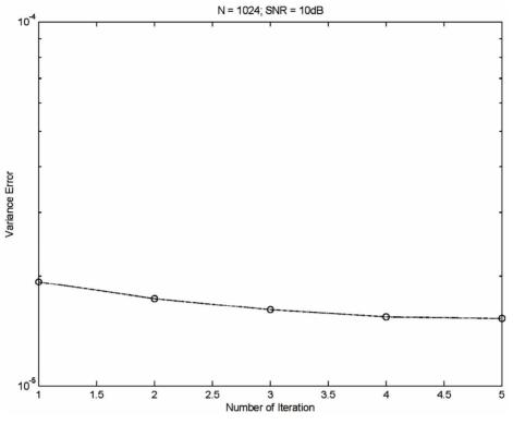
Figure 6. Frequency offset estimation with MAI elimination by using SIC.
