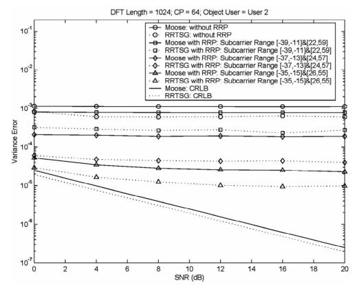
Figure 9. Performance comparison between Moose algorithm and the proposed RRTSG-based algorithm in heavy MAI environment.
