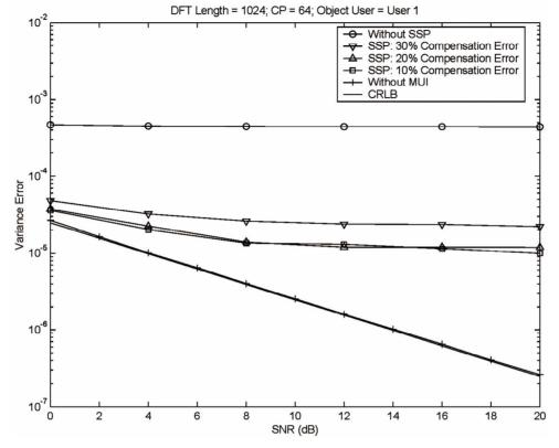
Figure 8. Frequency offset estimation with the help of heavy MAI elimination by using SSP.
