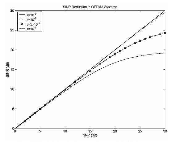
Figure 2. SINR reduction introduced by non-zero frequency offset in OFDMA systems.
