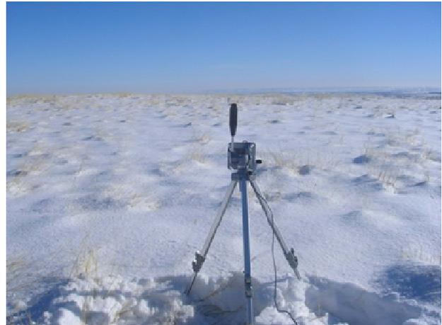
**Figure 3. Snow-covered crested wheatgrass field. The antenna is mounted vertically on the tripod with  $h = 71.5$  cm. This photograph was taken on January 20, 2012.**
