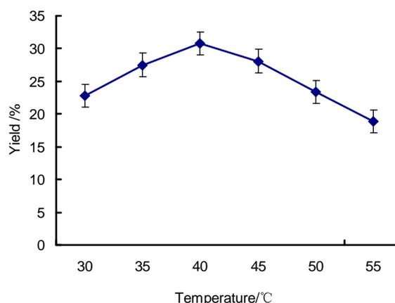
**Figure 2.** Effect of temperature on the reaction of sugar ester.
