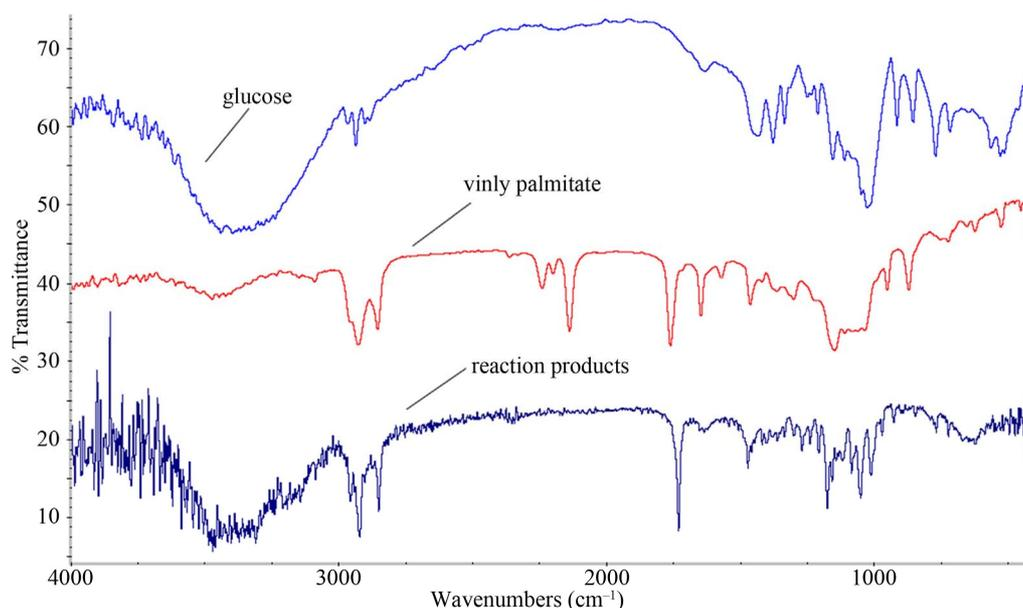
**Figure 5.** The FT-IR spectrum of glucose, vinyl palmitate and reaction products.
