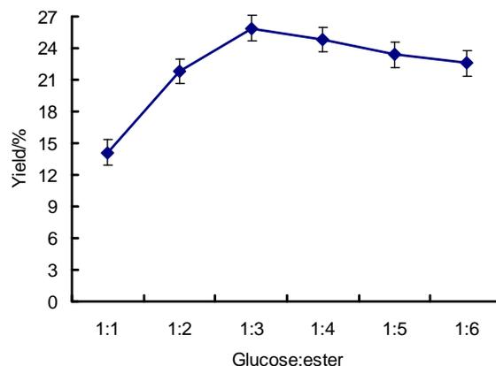
**Figure 3.** Effect of molar ratio of vinyl palmitate to glucose on the reaction of sugar ester.
