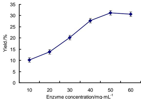
**Figure 4.** Effect of enzyme concentration on the reaction of sugar ester.
