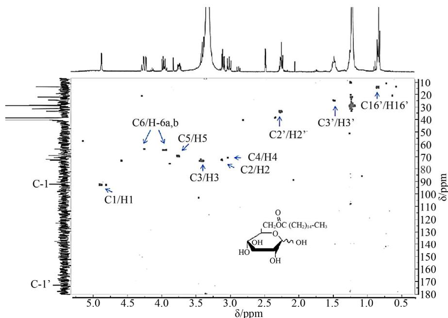
**Figure 8.**  $^1\text{H}$ - $^{13}\text{C}$  HSQC of the synthetic products in  $\text{CD}_3\text{OD}$  and  $\text{DMSO-d}_6$ .
