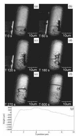
Figure 3. Snapshots of nano scratching using a hard cantilever tip (a)-(f) and the AFM profiles of the first scan (g). The time period of the images was 60 s (b), 120 s (c), 180 s (d), 270 s (e) and 600 s (f) after the LCM-DIM observation started (a). The AFM scan was repeated 40 times. After scanning, the cantilever stayed on the surface for 2 min (b) and (c) and moved away from the crystal. After scratching, the ditch was buried by the growing steps (c)-(f).
