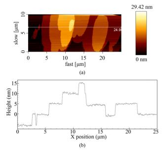
Figure 2. AFM image of the  $\{110\}$  surface (a), which is the same as that shown in Figure 1 and the height profile (b) indicated by the white line in Figure 2(a).
