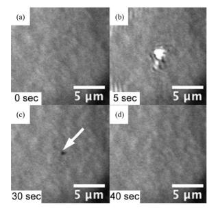
Figure 4. Time series images of the indentation by the AFM tip and its recovering. The images are taken every 5 s and the tip was approached for 20 - 30 s. They are typical images of (a) a flat surface before tip approaching; (b) the tip approaching on the surface; (c) a small hole on the surface after the tip retracted; and (d) the recovered flat surface.
