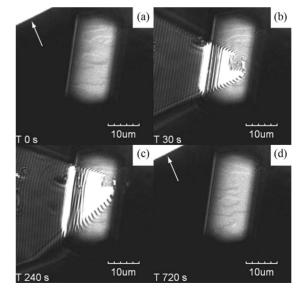
Figure 1. Snapshots of LCM-DIM images of HEW lysozyme crystal growth with an AFM cantilever tip. Two-dimensional nucleus steps grew on the {110} surface of HEW lysozyme in a supersaturated solution. The cantilever tip at the upper left is shown by arrows before (a) and after (d) AFM scanning. During the AFM observation (b) and (c), the cantilever was distorted because of image lag.
