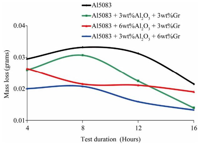
Figure 9. Effect of test duration in salt spray test.
