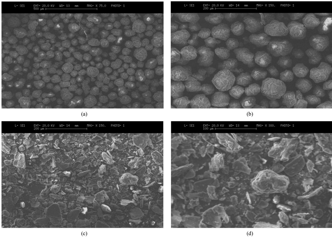
**Figure 1.** Scanning electron micrographs of  $\text{Al}_2\text{O}_3$  (a) and (b) and graphite (c) and (d).
