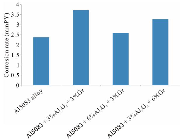
**Figure 12.** Effect of corrosion rate on samples prepared.
