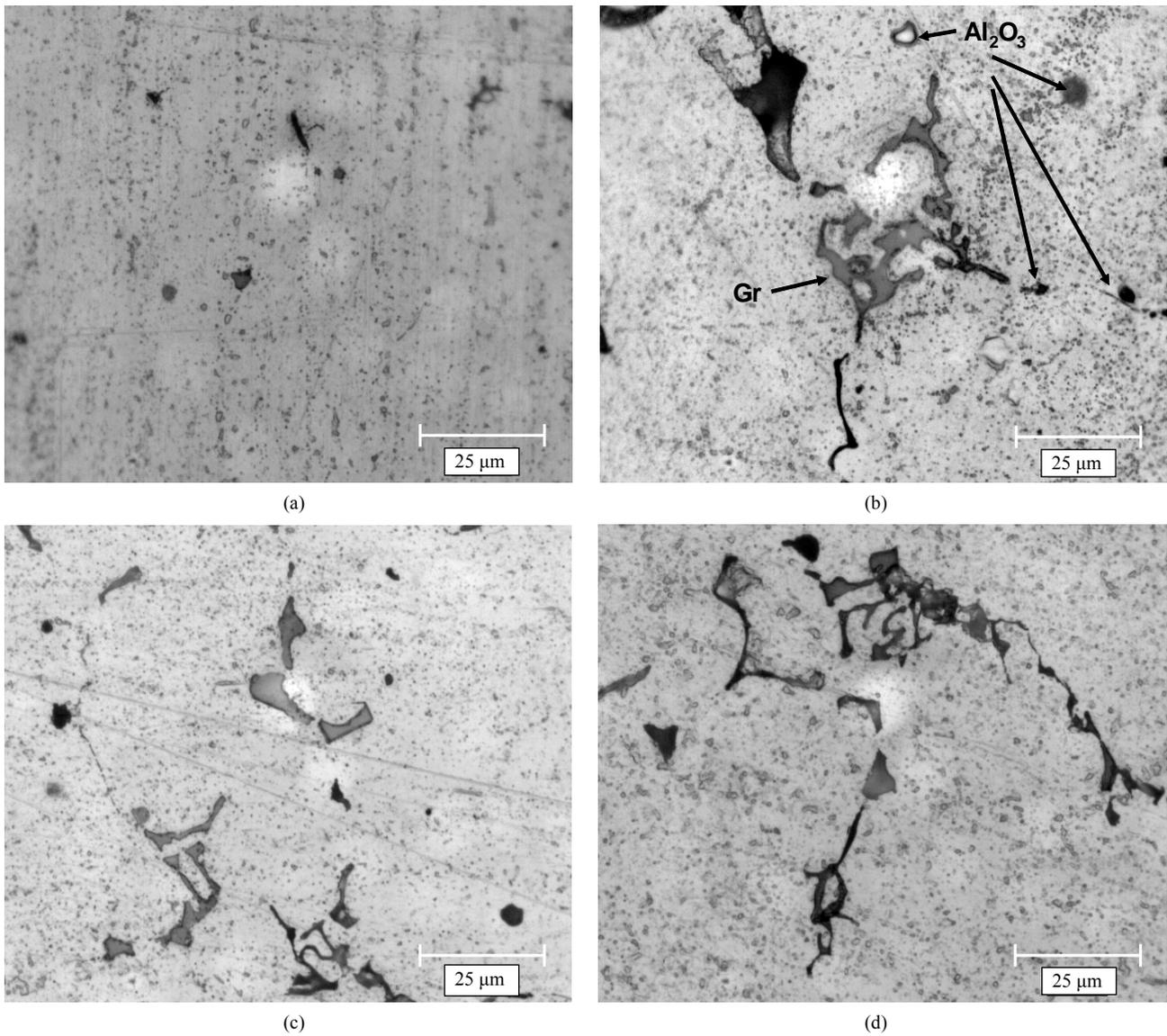
**Figure 2. Optical microstructure of composites.** (a) Al5083 alloy; (b) Al5083 + 3%Gr + 3%Al<sub>2</sub>O<sub>3</sub>; (c) Al5083 + 6%Gr + 3%Al<sub>2</sub>O<sub>3</sub>; (d) Al5083 + 3%Gr + 6%Al<sub>2</sub>O<sub>3</sub>.
