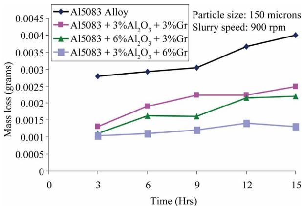
Figure 6. Effect of test duration on slurry wear.
