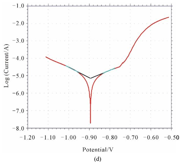
Figure 10. Polarization scan generated in potentiostat. (a) Al5083 Alloy; (b) Al5083 + 3%Al<sub>2</sub>O<sub>3</sub> + 3%Gr; (c) Al5083 + 3%Al<sub>2</sub>O<sub>3</sub> + 6%Gr; (d) Al5083 + 6%Al<sub>2</sub>O<sub>3</sub> + 3%Gr.
