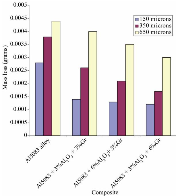
Figure 4. Effect of reinforcement of composites on slurry wear.
