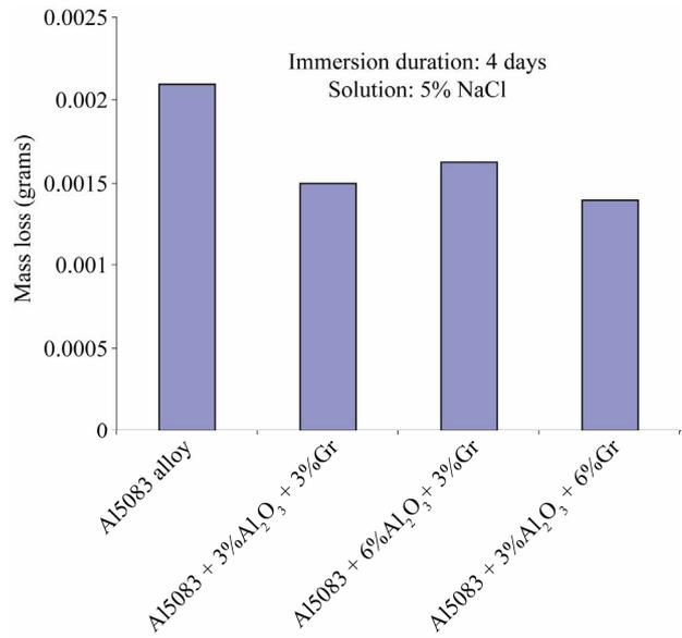
Figure 7. Effect of reinforcement in immersion test.
