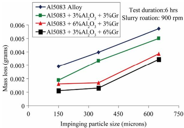
Figure 5. Effect of impinging particle size on slurry wear.
