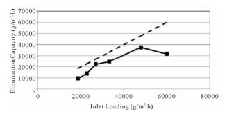
Figure 3. Elimination capacity in various inlet loading.
