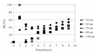
Figure 4.  $N_2O$  removal efficiency at various depths (filter medium = dry compost).
