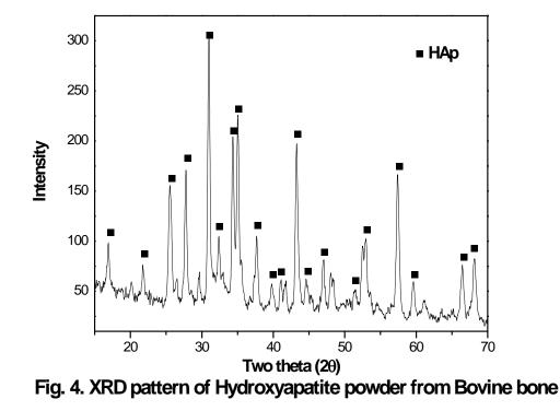
The Bragg reflection at (002) planes of HAp was considered to calculate the crystallite size. Crystallite size for HAp synthesized from fish scales and bovine bones are 69.6 nm, 77.62 nm respectively.
