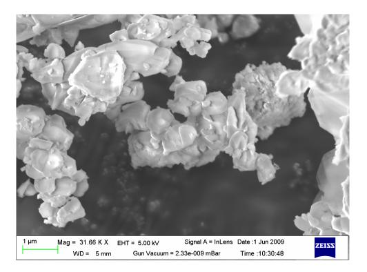
Fig.7. FE-SEM of HAp powder synthesized from Fish Scale
