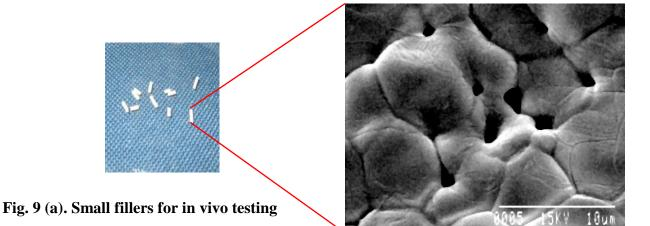
Fig. 9 (b). SEM image of the small fillers
