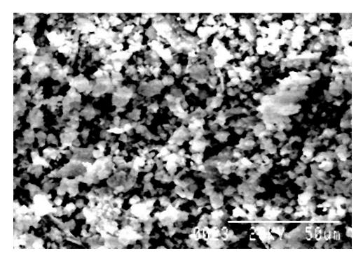
Fig. 8. FE-SEM of HAp powder synthesized from Bovine Bone
