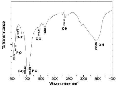
Fig. 6. FTIR spectrum of Hydroxyapatite powder from Bovine bone
