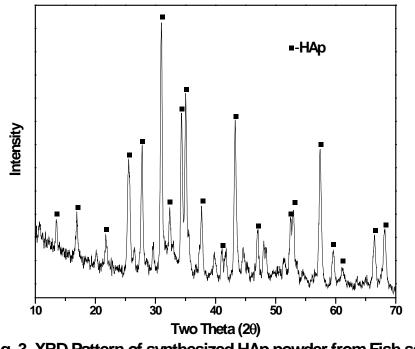
Fig. 3. XRD Pattern of synthesized HAp powder from Fish scale
