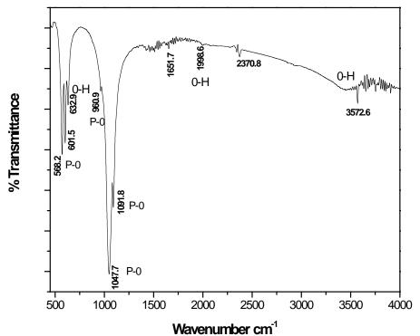
Fig. 5. FTIR Spectrum of Hydroxyapatite powder from Fish scale
