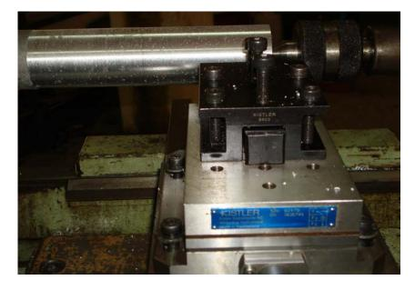
Figure 5 photographic view of experimental set up with kistler dynamometer
