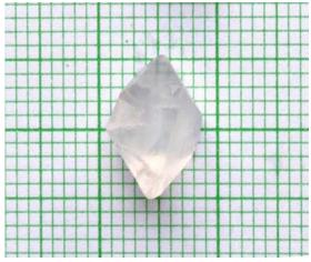
Fig .1. The grown single crystal of TGZC
