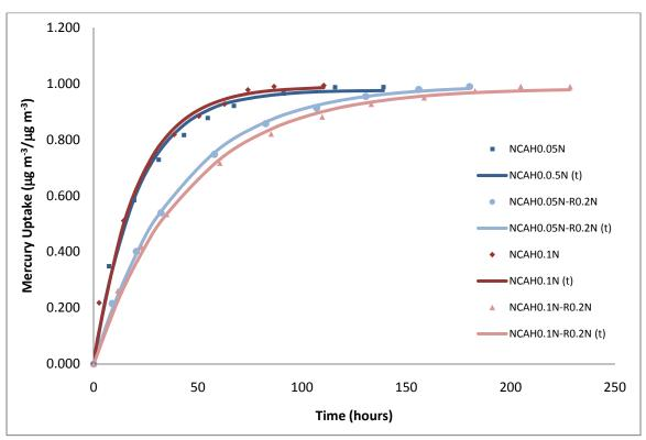
Figure 4: Regeneration of acidulated bamboo derived sorbents without epidermal tissue using low HCl concentrations
