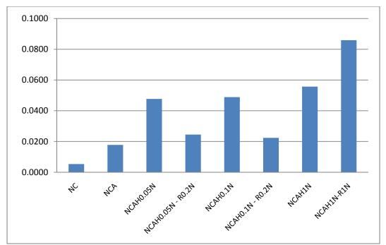
Figure 8: Rate Constants for mercury uptake by bamboo derived sorbents with skin with various treatments
