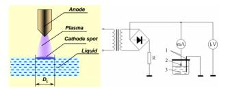
Figure 1. The scheme of atmospheric pressure glow discharge with electrolyte cathode.  $D_c$ —cathode spot diameter. 1—electrodes; 2—discharge zone; 3—solution under treatment.
