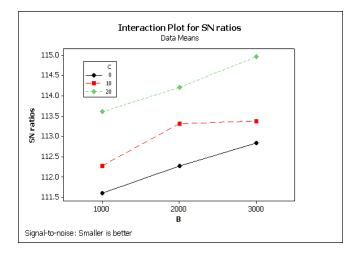
Figure 4 (c) Interaction graph for BXC for Specific wear rate.
