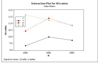
Figure2 (c) Interaction graph for BXC for Coefficient of friction
