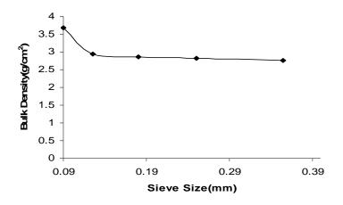
Figure 2. Variation of Bulk Density with Sieve Size.
