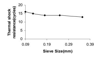
Figure 5. Variation of Thermal Shock Resistance with Sieve Size.
