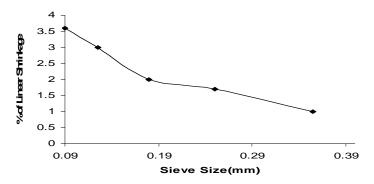
Figure 3. Variation of Linear Shrinkage with Sieve Size.
