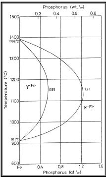
Fig 4: High temperature gamma loop region of the Fe-P phase diagram (Kubaschewski 1982)
