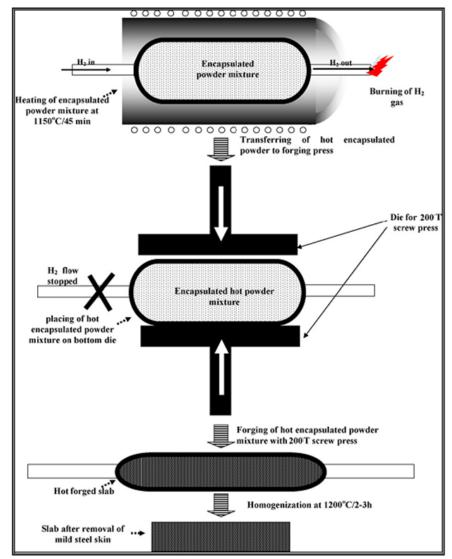
Fig.2: Schematic diagram illustrating the production of slab by hot forging of encapsulated powder mixture.
