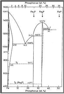
Fig 3: Fe–P binary phase diagram (Kubaschewski 1982).
