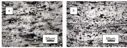
Fig 8: Microstructures of rolled and annealed alloys etched with 2% Nital. Pores are elongated in the rolling direction. (a)Sample 2 & (b) Sample 3.
