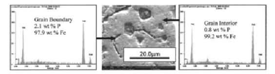
Fig 9: Surface morphology and EDAX pattern from different spots on Sample 2
