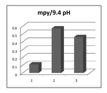
Fig 7: Bar chart displaying corrosion data (Linear Polarization) for Phosphoric irons in 0.5M Na<sub>2</sub>CO<sub>3</sub> + 1.0 M NaHCO<sub>3</sub> solution (9.4 pH)
