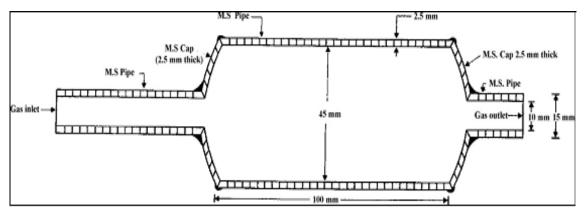
Fig.1: Cross-section of mild steel capsule used in the present investigation.
