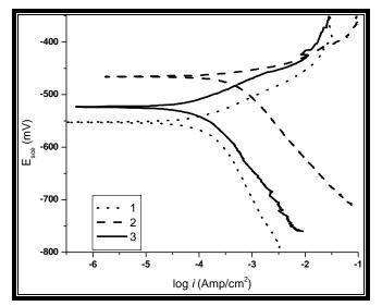
Figure 5: Tafel curves for Phosphoric irons in 0.25 M H<sub>2</sub>SO<sub>4</sub> solution (0.6 pH).
