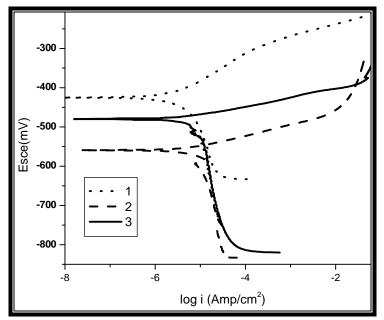
Figure 6: Tafel curves for Phosphoric irons in 3.5 % NaCl solution (6.8 pH)
