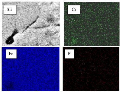
Fig 11: Composition Image [Secondary Image] & X- Ray Mapping of Sample 3.
