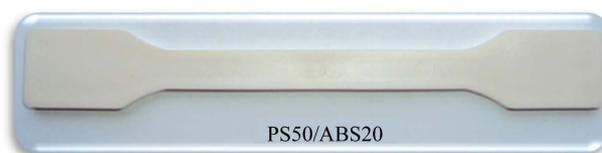
**Figure 1.** Injection molded sample of PS50/ABS20 blend.
