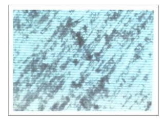
Plate8. 90% Deformation, 380°C, 30min
