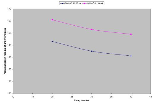
Figure 2. Effect of holding time on recrystallization rate at constant temperature (450°C).
