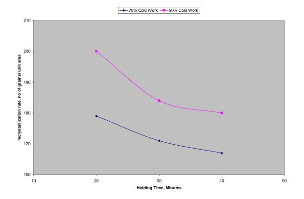
Figure 1. Effect of holding time on recrystallization rate at constant temperature (380°C).
