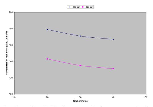
Figure 3. Effect of holding time on recrystallization rate at constant %cold deformation (70%)
