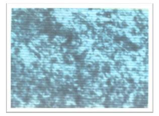
Plate 7. 90% Deformation, 380°C, 20min
