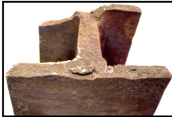
Figure 1. Fracture surface of one of the samples-HK-40.
