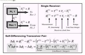
Fig. 5 Double differencing with transceivers (LeMaster, 2002)
