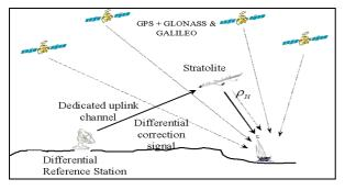
Fig. 1 Differential satellite positioning with a stratolite (http://www.helinet.polito.it)
