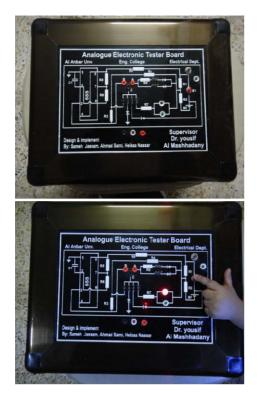
Figure 4. The practical model of electronic tester board.
