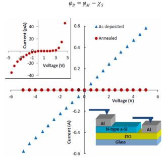
Figure 5. Current-voltage characteristics of ITO/n-type a-Si:H thin film junctions after deposition and annealing. The as-deposited n-type Si film shows ohmic contact with ITO. After annealing, the contact deteriorates to a Schottky type contact with increased contact resistance. The top inset shows the current-voltage characteristics of the annealed sample. The bottom inset shows the schematic of the sample used for the measurement.
