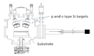
Figure 1. Schematic of the AJA Orion 1800F RF/DC Sputter deposition system used to deposit thin films of p- and n-type a-Si:H on ITO/Glass substrates.
