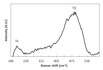
Figure 2. Raman spectroscopy scan of as-deposited p-type a-Si:H film. The peaks at 160 and 480 cm<sup>-1</sup> correspond to amorphous Si-Si transverse acoustic (TA) and transverse optic (TO) vibrational modes, respectively.
