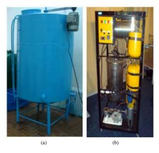
Figure 4. (a) A 2 ton biodiesel processor and (b) A glycerol purification system [11,90].
