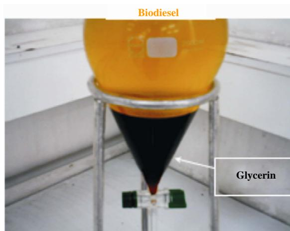
**Figure 5. Biodiesel and glycerin separation [4].**
