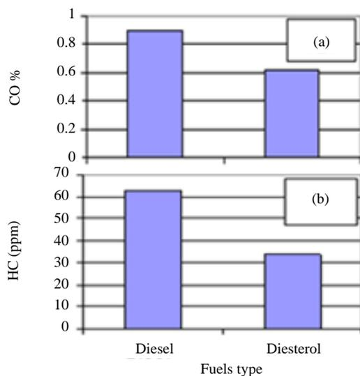
Figure 8. (a) CO and (b) HC emissions of diesel and diesterol fuels at engine full load [74,86].
