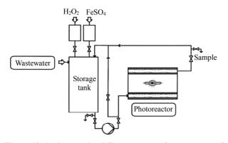
Figure 12. A photo assisted Fenton system for treatment of pesticide wastewater [70].
