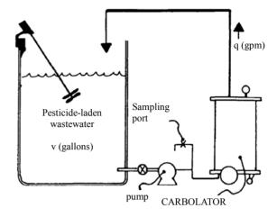
Figure 16. Recirculation through activated carbon [103].
