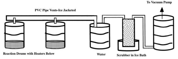
Figure 14. A KPEG process with vent system [86].
