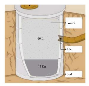
Figure 4. A cross section of a plastic pit for disposal of pesticide wastewater [40].
