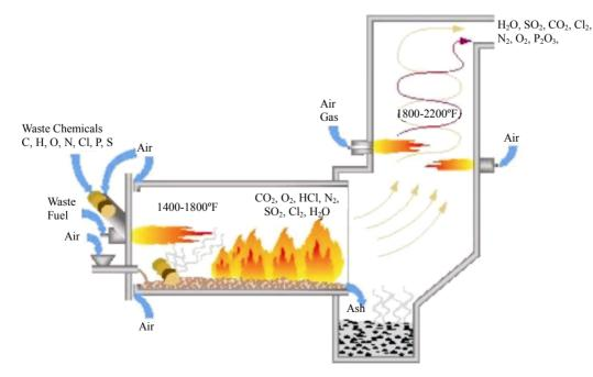
Figure 9. An incinerator for pesticide wastes [61].
