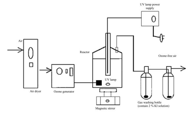
Figure 11. A UV/O<sub>3</sub> system for the treatment of pesticide wastewater [68].
