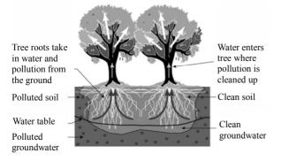
Figure 17. Phytoremediation to clean up pesticide contaminated grounds [1].
