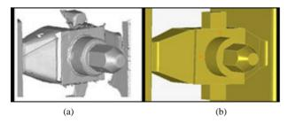
Figure 2. Use of industry standard (a) 3-D laser scanner and (b) CAD software on Laser Scanner (Source: [13]).
