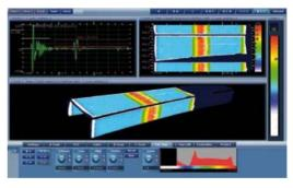
Figure 3. C-Scan map of a composite spar structure displayed on 3D image (Source: [16]).
