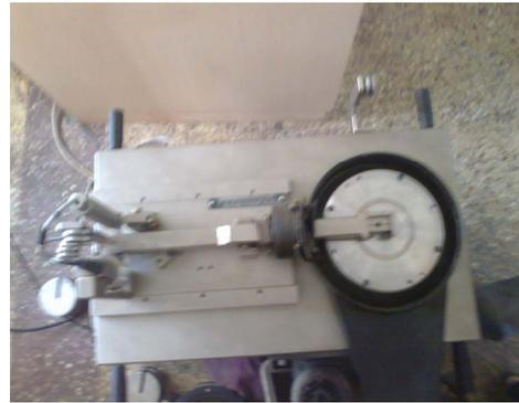
**Figure 6. Wear and friction test rig.**
