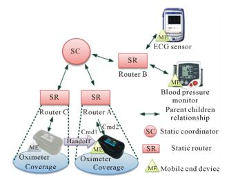
Figure 1. ZigBee Fixed-Mobile Network (ZFMN).
