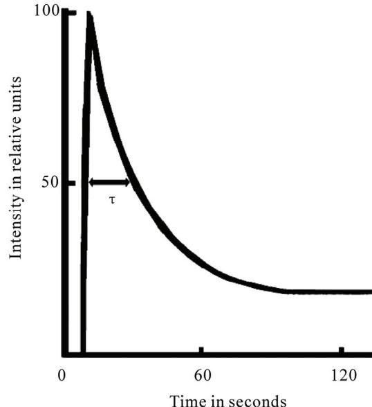
**Figure 1.** Induction curve of delayed fluorescence of chlorophyll.
