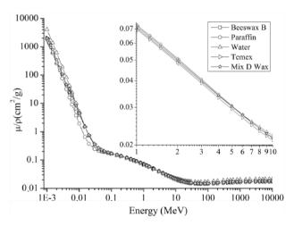
Figure 4. Comparison of the behavior of the mass attenuation coefficients (obtained using the program Xcom) of beeswax B with other simulators.
