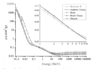
Figure 5. Comparison of the behavior of the mass attenuation coefficient (obtained using the program Xcom) of beeswax B with main body tissues.
