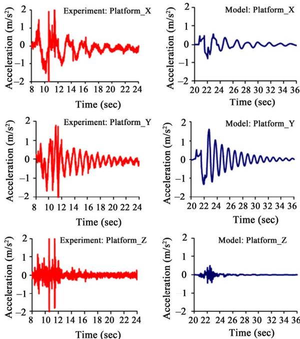
**Figure 6.** Comparisons of the modeling and experimental responses of the scissor lift to the pothole depression under the test conditions: fully-elevated platform, pulled-out extension, and fully-loaded.
