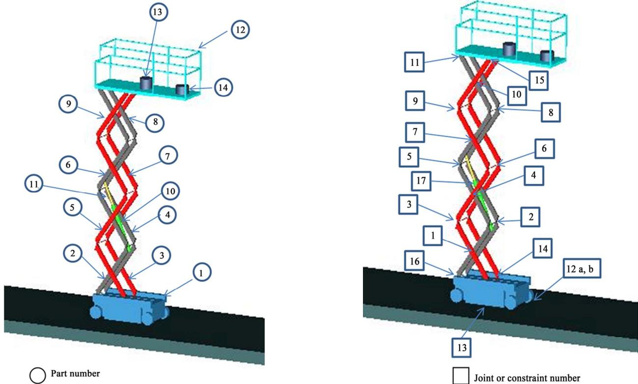
**Figure 3.** An ADAMS model of the scissor lift.
