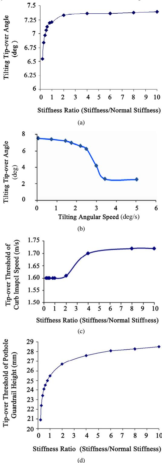
**Figure 7.** The tip-over thresholds under four hazardous conditions. (a) The effect of the structure stiffness of scissor lift on the quasi-static tip-over threshold (tilt angle). (b) The effect of tilt speed on the tip-over threshold (tilt angle). (c) The effect of curb impact speed on the tip-over. (d) The effect of scissor structure stiffness on the requirement of the guard-
