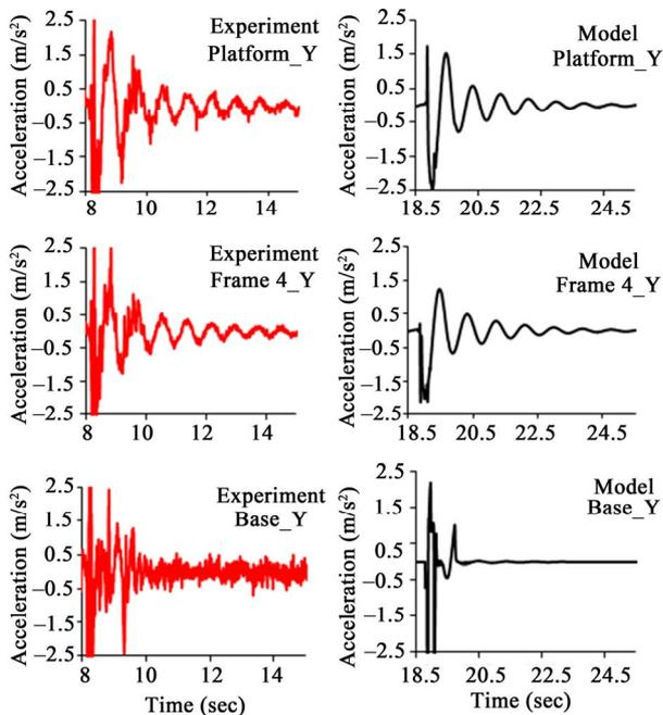
**Figure 5.** Comparisons of the modeling (right column) and experimental responses of the scissor lift to the 90° curb impact under the test conditions: fully-elevated platform, no extension, and fully-loaded.
