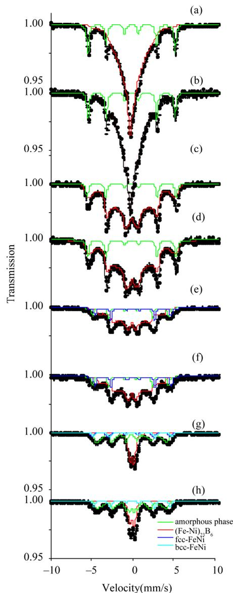
**Figure 2.** Spectra of nanocrystalline Fe-Ni-Nb-B alloys, where (a) and (b) corresponds to 1:0 ratio of Fe:Ni; (c) and (d) to 3:1; (e) and (f) to 1:1; (g) and (h) to 1:3. The spectra (b), (d), (f) and (h) were taken in the weak external magnetic field.
