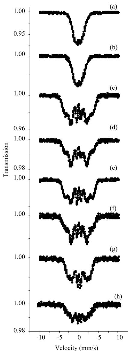
**Figure 1.** Spectra of amorphous Fe-Ni-Nb-B alloys, where (a) and (b) corresponds to 1:0 ratio of Fe:Ni; (c) and (d) to 3:1; (e) and (f) to 1:1; (g) and (h) to 1:3. The spectra (b), (d), (f) and (h) were taken in the weak external magnetic field.
