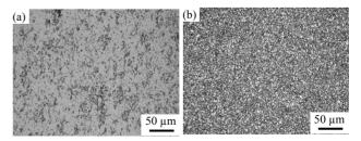
Figure 2. Microstructure of W70Cu30 wires after corrosion (a) tungsten (b) copper.
