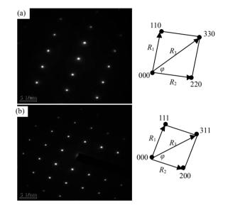
Figure 5. Diffraction pattern and calibrated graph of W70Cu30 wire before and after hot-swaging (a) A area; (b) B area.
