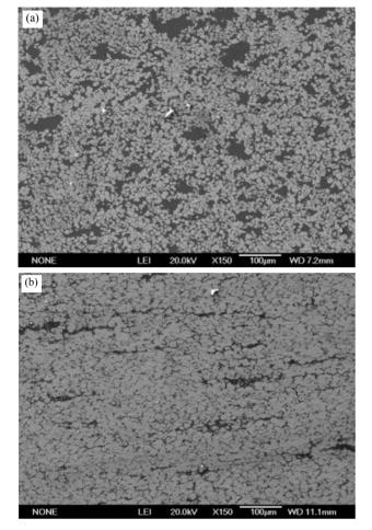
Figure 3. Microstructure of cross-section of W70Cu30 alloys before (a) and after (b) hot-swaging
