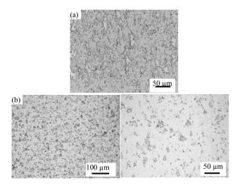
Figure 1. Microstructure of W70Cu30 wires before (a) and after (b) hot-swaging.
