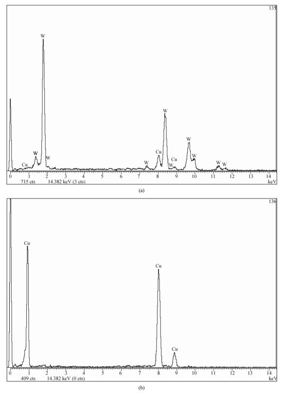
Figure 6. Spectrum diagrams of W70Cu30 wire before and after hot-swaging (a) A area; (b) B area.
