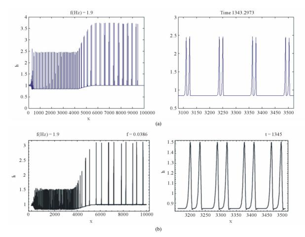
Figure 3. Wave profile in the forced film flow of the Newtonian fluid (n = 1, Re = 3.85, f = 0.0386, t = 1325): (a) Equation (5.1), We = 0; (b) Equation (5.2), We = 10.
