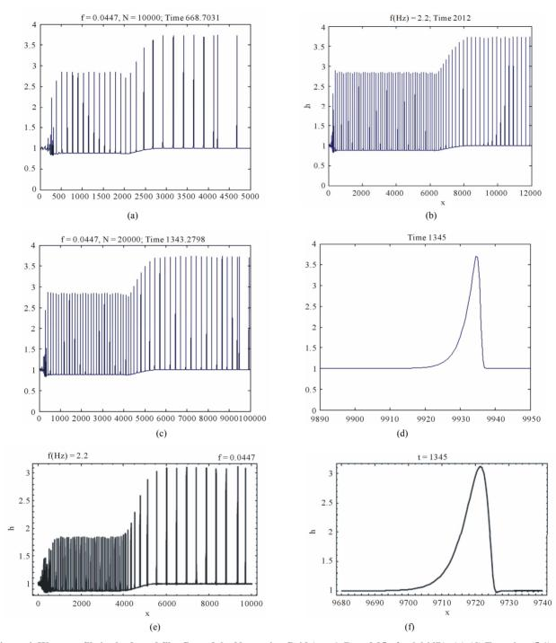
Figure 4. Wave profile in the forced film flow of the Newtonian fluid (n = 1, Re = 3.85, f = 0.0447): (a)-(d) Equation (5.1), We = 0; (e)-(f) Equation (5.2), We = 10; (a) t = 669; (b) t = 2012; (c)-(f) t = 1345.
