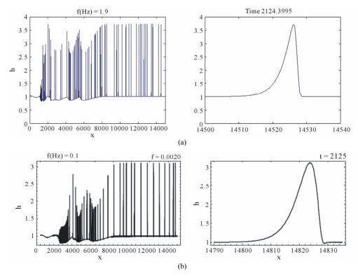
Figure 2. Wave profile in the forced film flow of the Newtonian fluid (n = 1, Re = 3.85, f = 0.002, t = 2125): (a) Equation (5.1), We = 0; (b) Equation (5.2), We = 10.
