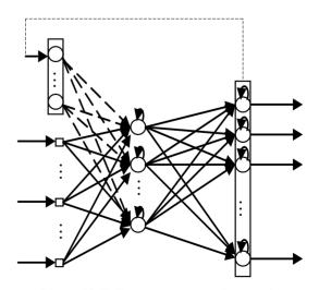
Figure 10. Fully recurrent neural network.
