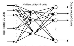
Figure 7. A three layers feedforward network.
