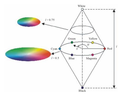
Figure 4. (Gonzalez [19]): The HSI color model based on circular color planes. The circles are perpendicular to the vertical intensity axis.
