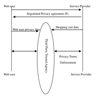
Figure 3. An example of a third party trusted agency acting as an intermediary between web user and service provider.
