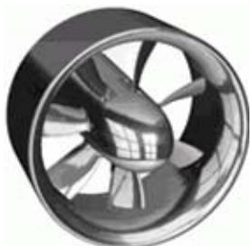
Figure 1. Engine type ducted fan.
