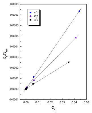
Figure 7. Langmuir isotherm for Sr<sup>2+</sup> ions on FAM sorbent at different reaction temperatures and at pH 4.
