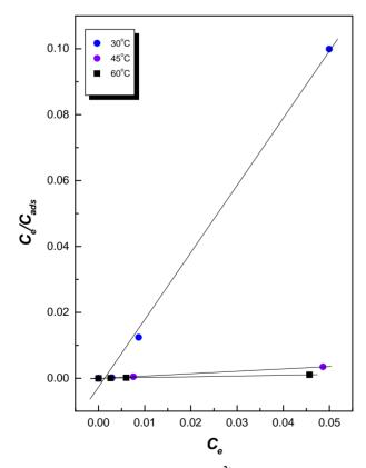
Figure 2. Langmuir isotherm for Co<sup>2+</sup> ions on SAM sorbent at different reaction temperatures and at pH 4.
