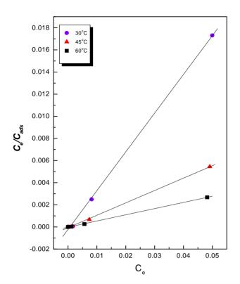
Figure 1. Langmuir isotherm for Cs<sup>+</sup> ions on SAM sorbent at different reaction temperatures and at pH 4.
