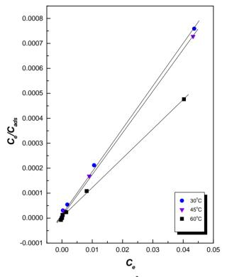
Figure 3. Langmuir isotherm for  $Sr^{2+}$  ions on SAM sorbent at different reaction temperatures and at pH 4.
