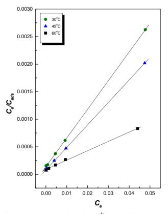
Figure 4. Langmuir isotherm for Cd<sup>2+</sup> ions on SAM sorbent at different reaction temperatures and at pH 4.
