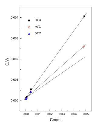
Figure 5. Langmuir isotherm for Cs<sup>+</sup> ions on FAM sorbent at different reaction temperatures and at pH 4.
