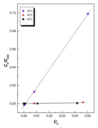
Figure 8. Langmuir isotherm for Cd<sup>2+</sup> ions on FAM sorbent at different reaction temperatures and at pH 4.
