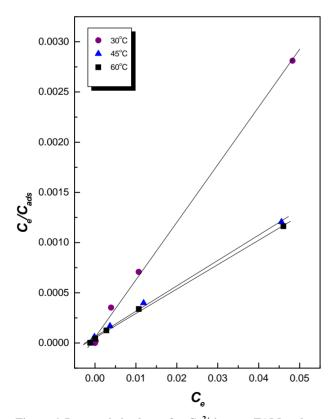
Figure 6. Langmuir isotherm for Co<sup>2+</sup> ions on FAM sorbent at different reaction temperatures and at pH 4.
