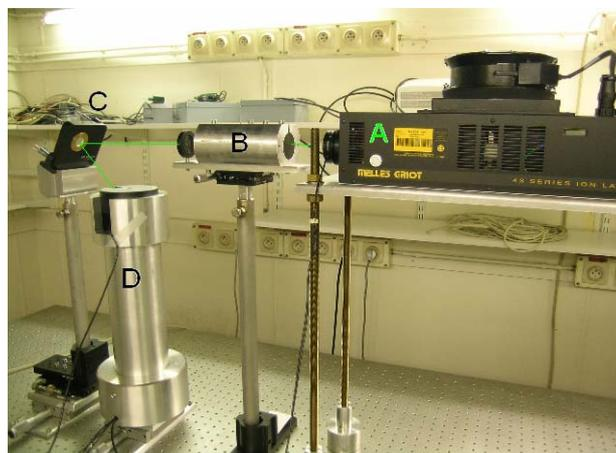
**Figure 1.** Layout of the OSL facility (A: Ar laser—B: Beam expander C: Mirror—D: tube with detector support, optics and PMT).
