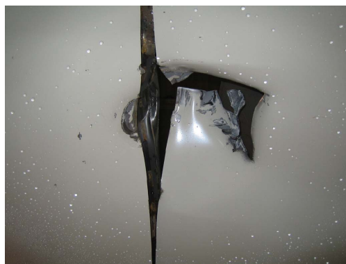
Figure 9. Broken roof of the protective box by the flying parts (Figure 5) in the fracture case of the vessel without outer cover.
