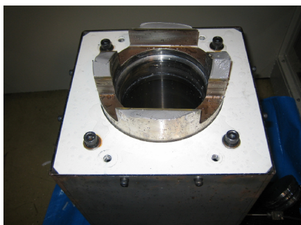
Figure 6. Remained parts of arm guide (The part shown in Figure 1). Fracture surface shows smooth brittle features.
