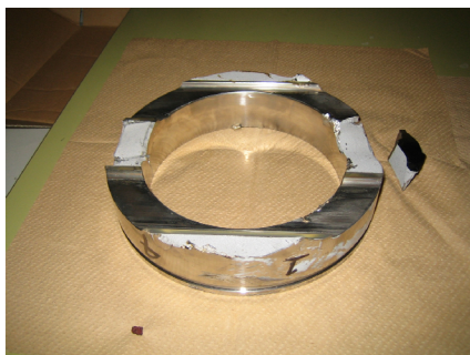
Figure 5. Flying parts of broken arm guide (The top part of Figure 1). Angle of fracture surface is about 45 degree (left and right side).
