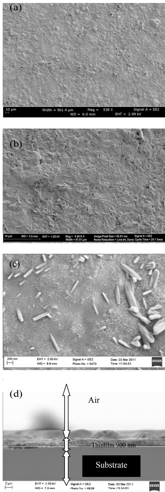
**Figure 2.** Top-view SEM images of CdS nanofilm at different magnification powers (a-c) and cross-section (d).
