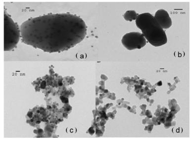
Figure 1. TEM images of Ag-TiO<sub>2</sub> composites (a) 1:10 Ag-TiO<sub>2</sub> R902; (b) 1:50 Ag-TiO<sub>2</sub> R902; (c) 1:10 Ag-TiO<sub>2</sub> P25; (d) 1:50 Ag-TiO<sub>2</sub> P25.
