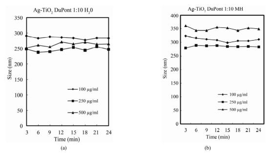
Figure 3. Temporal evolution of the Ag-TiO<sub>2</sub> DuPont 1:10 composite size (z-average): (a) deionized water; (b) Mueller Hinton Broth.
