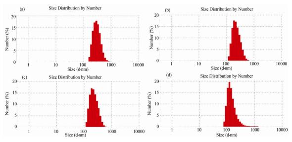
Figure 2. DLS results (a) 1:10 Ag-TiO<sub>2</sub> R902; (b) 1:50 Ag-TiO<sub>2</sub> R902; (c) 1:10 Ag-TiO<sub>2</sub> P25; (d) 1:50 Ag-TiO<sub>2</sub> P25.
