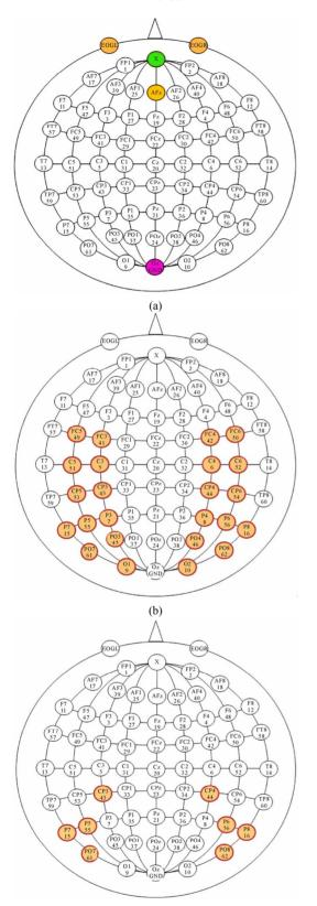
(c) **Figure 2.** Electrodes diagram (a) 62 channel; (b) 24 channel; (c) 8 channel.
