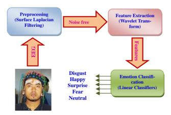
Figure 1. Basic emotion recognition system using EEG.
