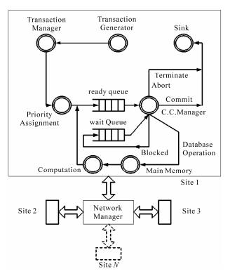
Figure 1. Distributed real-time database system model.
