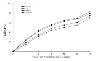
Figure 6. Miss % with (RC + DC) at communication delay 100ms normal and heavy load.
