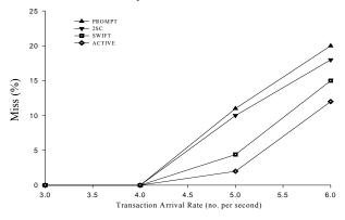
Figure 4. Miss % with (RC + DC) at communication delay 0ms normal load.
