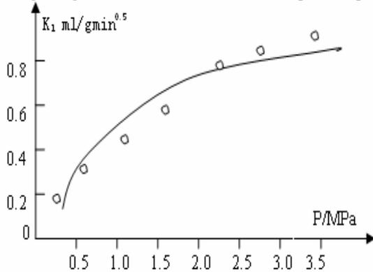
**Figure 1. Relation curve of the gas desorption index for drilling bits and the gas pressure P of 13-1 coal sample**
