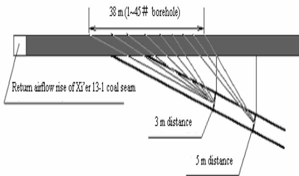
**Figure 2. The profile chart of drilling arrangement at 3 m and 5 m from crosscut to the coal seam floor**
